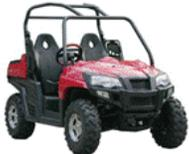
A side-by-side ATV has two abreast seats, typically built with a hood, and uses a steering wheel instead of a motorcycle steering handlebar.
