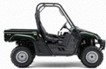
A utility terrain vehicle (UTV) has similar characteristics to a side-by-side ATV, but typically also features a box bed. UTVs are generally designed for utility rather than for recreational purposes.
